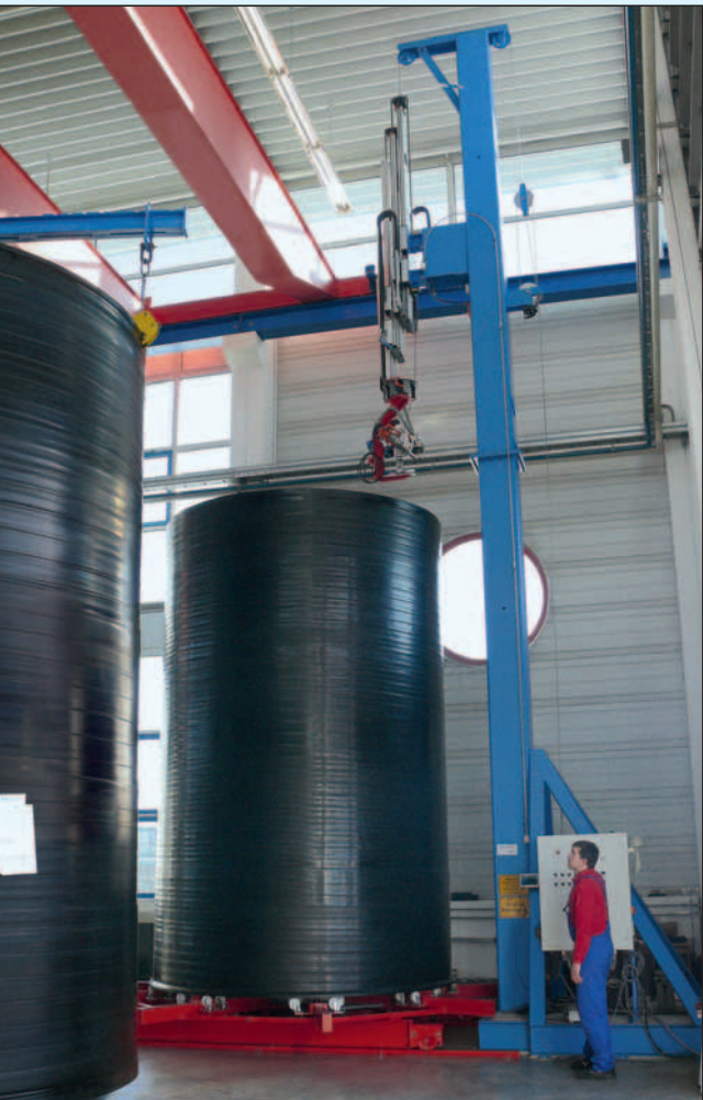
Automatic Extrusion Welding Machine. Bottoms can be welded to the shells
