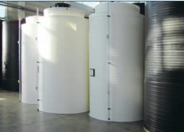
Storage Container fabricated from natural-coloured HDPE (Foods grade)
