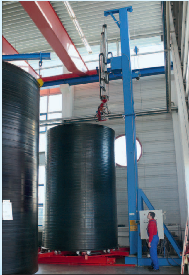
Automatic Extrusion Welding Machine. Bottoms can be welded to the shells
